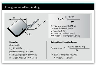
Bending force required when bending Quard 400, 450 and Quend 700 plates in lengths of 2,500 mm shown in plate thickness.
